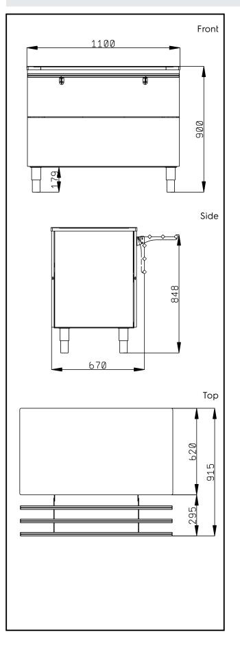
Flexy Compact Ambient Unit on cupboard (3 GN) with one stainless steel tray slider
